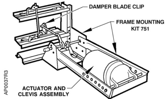
**Figure 3. One-section Damper.**
