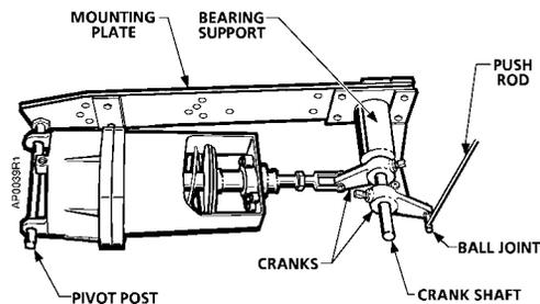
**Figure 9. Extended Shaft Remote Mounting Assembly.**
