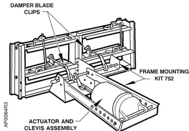
Figure 5. Two-section Damper.
